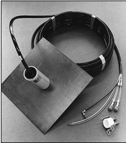
Settlement cell with plate, tubing, and reservoir.
